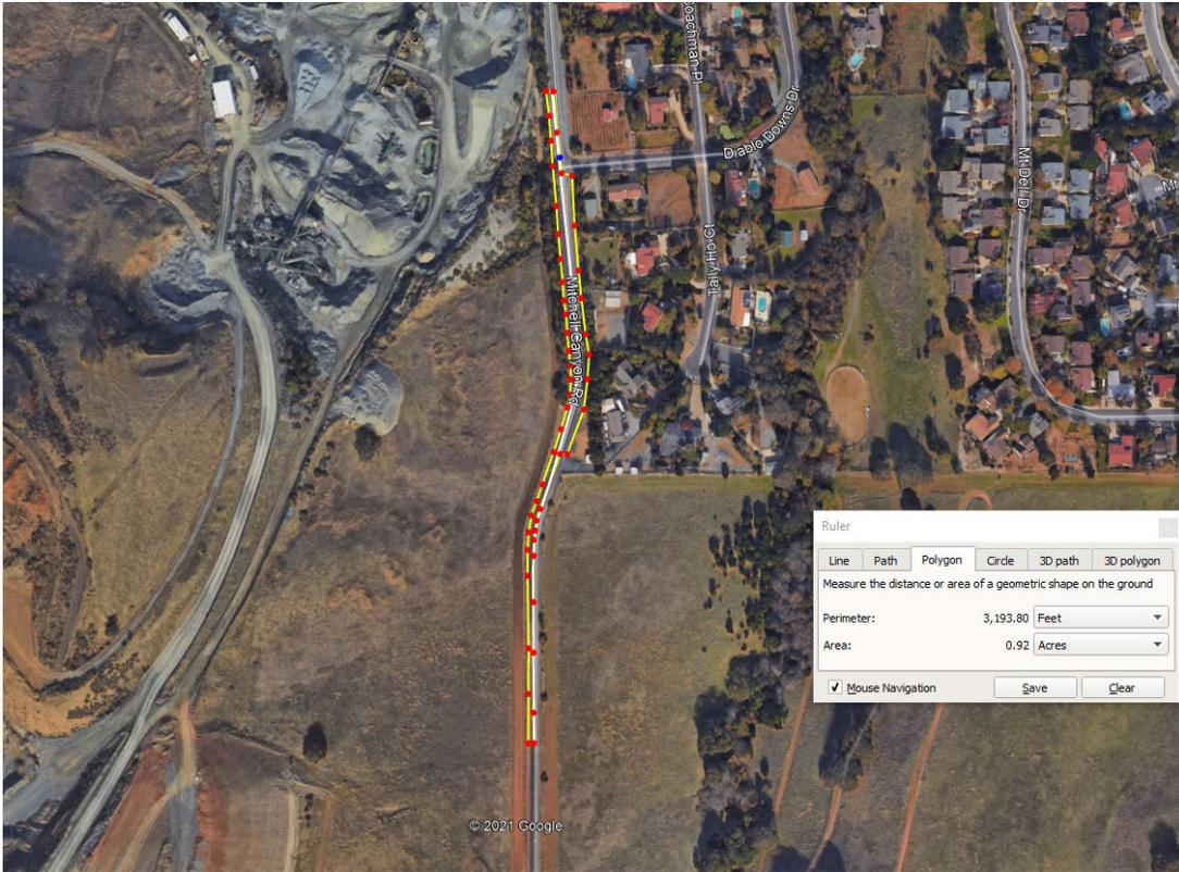
**Figure 2. Area of Mitchell Canyon Road Draining to 15-inch RCP in DA71A**
