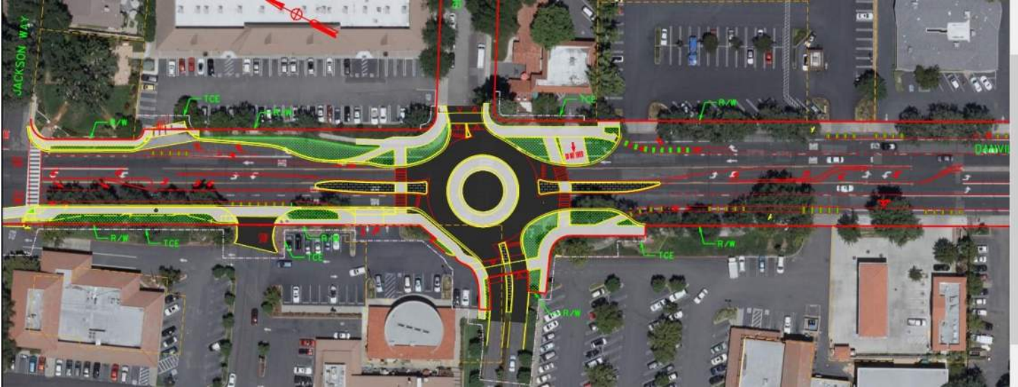
Figure 1. Plan View of the new roundabout at Danville Boulevard. and Orchard Ct.
