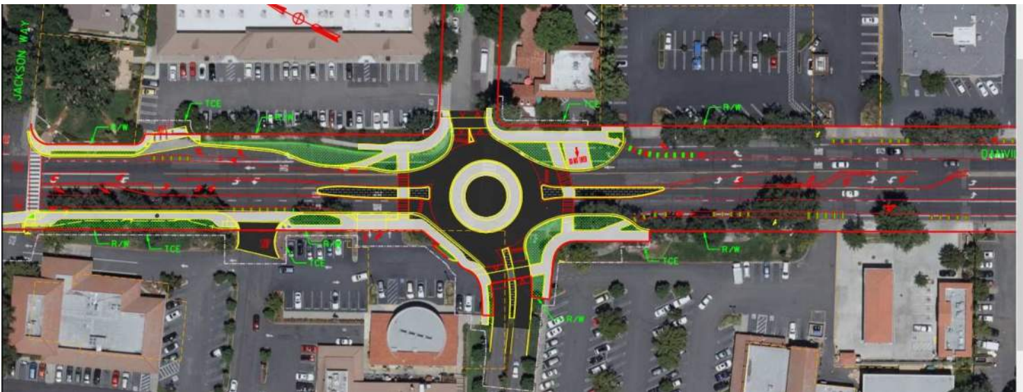
Figure 2. Plan View of the new roundabout at Danville Boulevard. and Orchard Ct.
